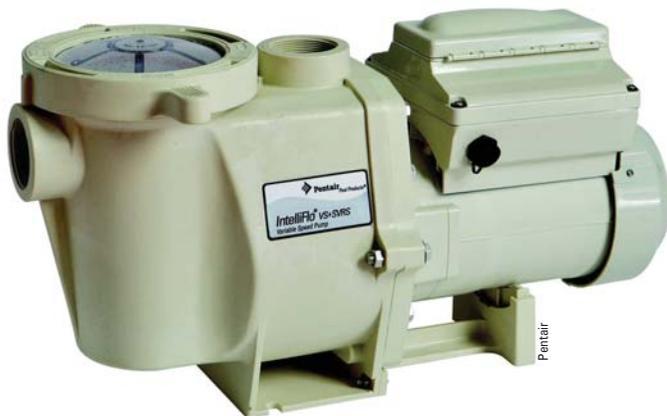
Since you cut the flow in half you now have to run the pump twice as long to get the same filtration. But the net result is you are using ¼ of the energy compared to an outdated pool pump. Bottom line—you run your pump at a slower speed for longer periods of time, but it's far more efficient and costs less to operate. Also variable speed pumps are higher quality motors, so they last longer. Manufacturers estimate a 15 year life, based on advanced aging tests.
