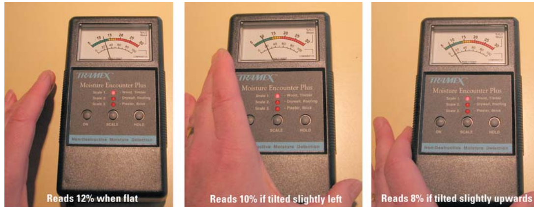
Figure 3. A technician's skill can significantly influence the meter reading
