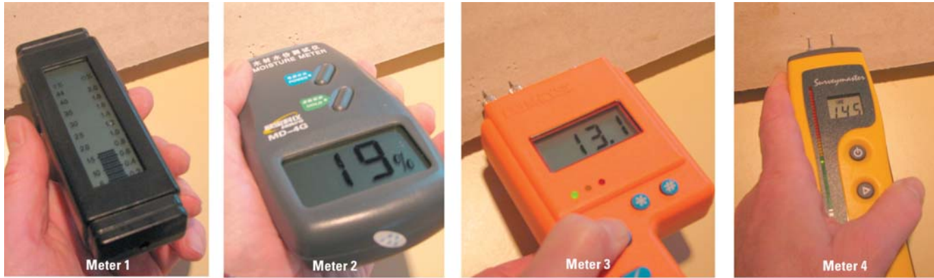
Figure 4. Meters from different manufacturers show different values for “saturated” moisture content
