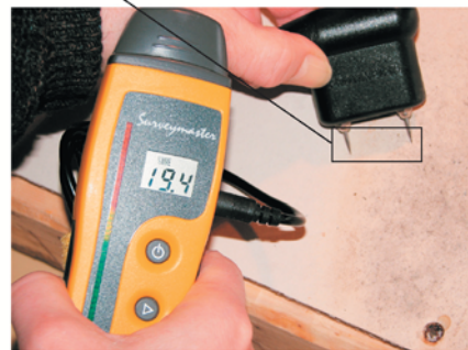
Figure 1. Moisture content and therefore mold growth can vary significantly over short distances
