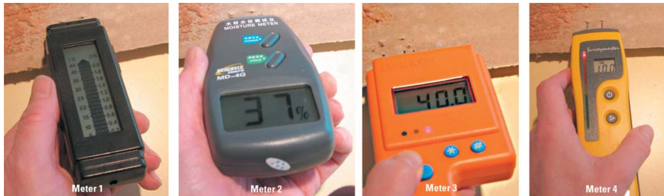
Figure 5. Different meters also show different values in the range of mold-risky moisture contents
