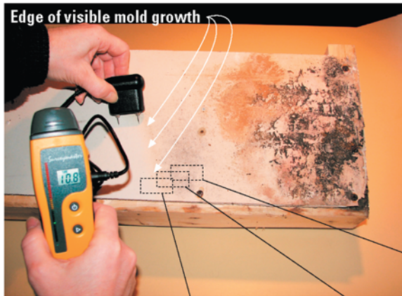
Figure 1. Moisture content and therefore mold growth can vary significantly over short distances
