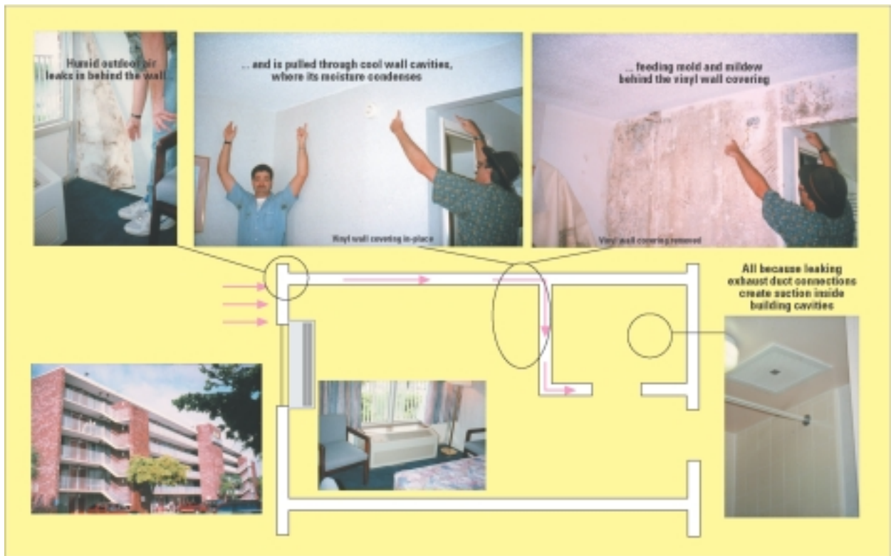
Figure 12. Leaking HVAC duct work pulls humid air into a building to support mold growth.
